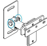
b) Turn the speaker holding plate with attached T-plate aside so that you will be able to mount the speaker easily.
