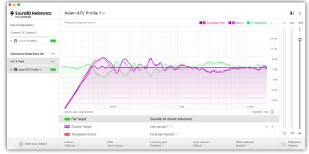
Sonarworks SoundID correction curves can be uploaded directly to the A7V.
