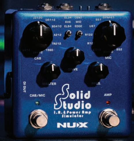
IR Loader with built-in cabinet, microphones and microphone positions, power amp simulator with 3 tubes, power amp controls
