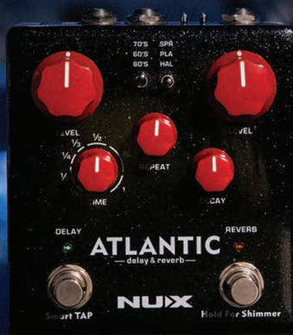
Multi Delay and Reverb effect pedal with inside routing and secondary reverb effects
