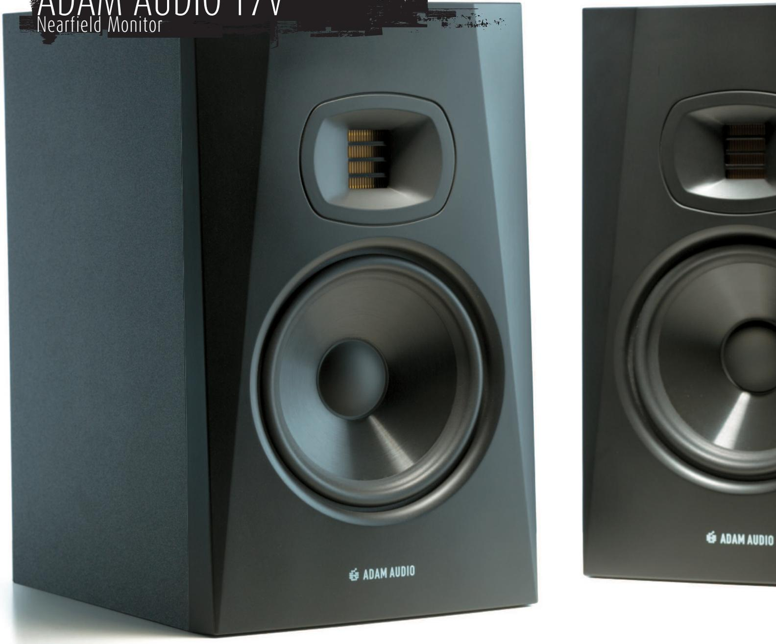
In the 07/08.2017 issue of Sound & Recording, we reviewed the new S-series monitor by ADAM Audio, the S3V. The Berlin-based company latest release is the T-series, positioned considerably below the S-series in terms of features and price yet offering some impressive characteristics such as a U-Art Air Motion Transformer for the tweeter, a DSP system and newly developed Class D power amps.
